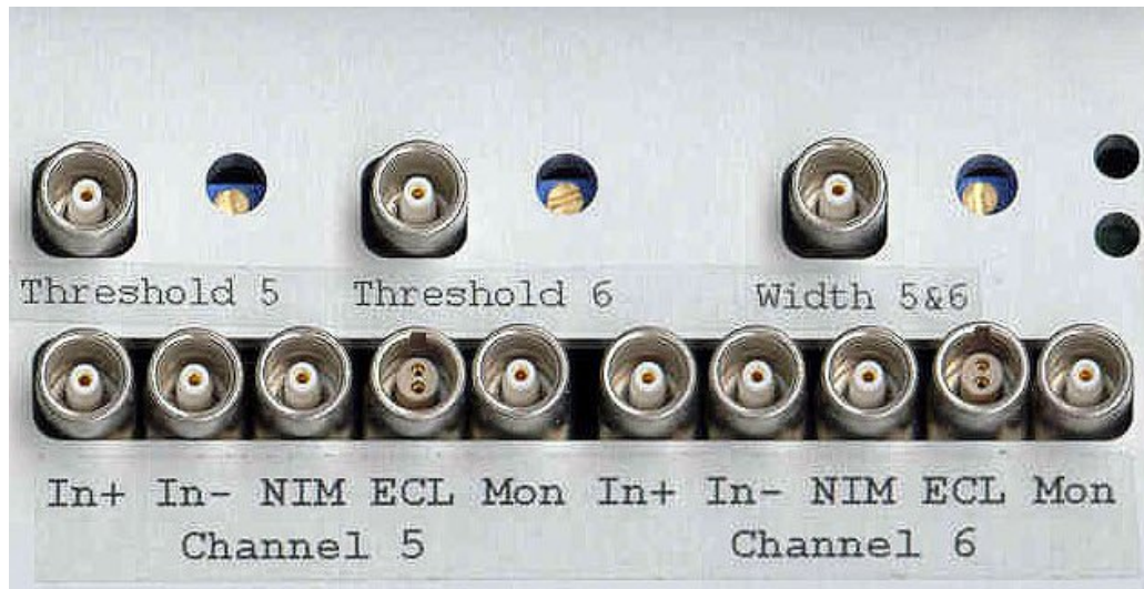
Figure 2.35: inputs, outputs and controls of the ATR19 for each internal DLATR board
