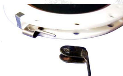
Figure 2.15: MCP stack with spring ring for MCP back cable (DLD40, DLD80 & HEX80)
